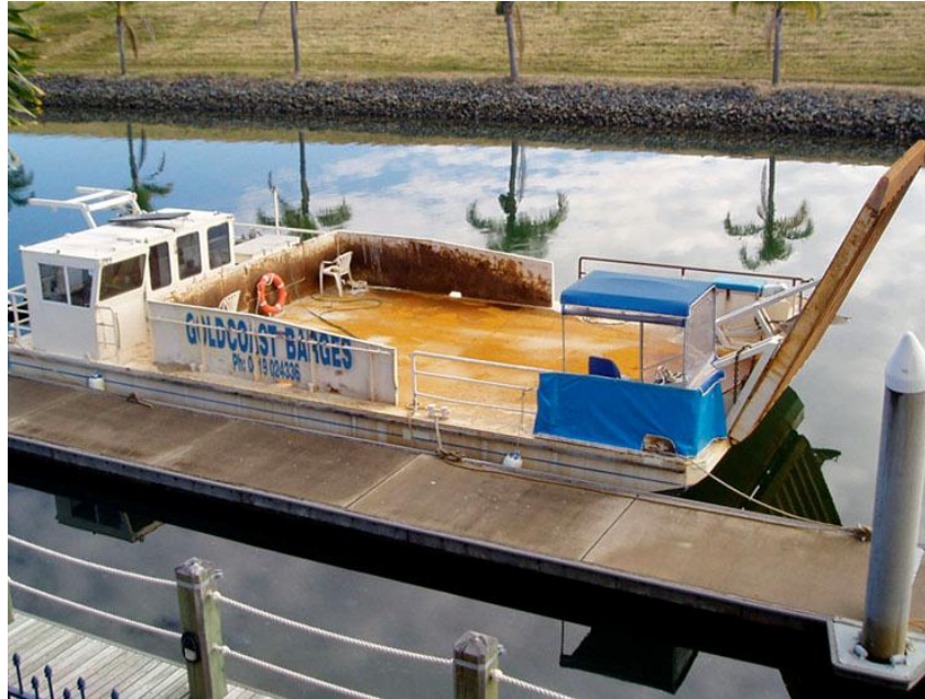
(12m Work / Landing Barge)
